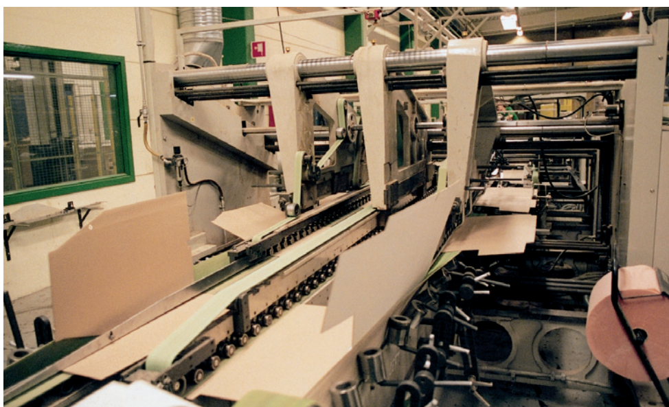
The DIBP issue particularly concerns adhesives used at the folder gluer machine stage
