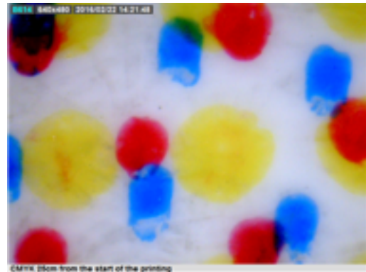
Cyan dots stretched in print direction
